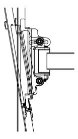
Loosen the clamping knobs that lock the tilt angle adjustment, then position the TV at the desired angle and tighten the terminal knobs to lock the TV in its position.
